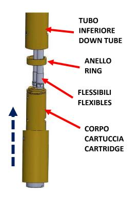
3) AVVITARE I 2 FLESSIBILI NEL CORPO CARTUCCIA, INFILARLI NELL'ANELLO E NEL TUBO INFERIORE SCREW THE 2 FLEXIBLES ON THE CARTRIDGE BODY, PUT THEM IN THE RING AND IN THE DOWN TUBE
