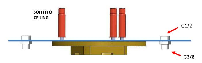
2) FISSARE CON I 3 TASSELLI LE PIASTRE AVVITATE E INSERIRE I 2 RACCORDI PER I FLESSIBILI CON VALVOLA DI NON RITORNO, IN DOTAZIONE, NELLE RELATIVE PRESE D'ACQUA G1/2.
